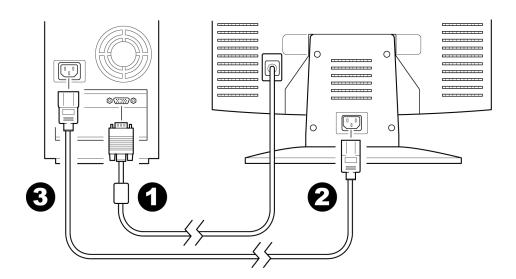
The power cord supplied with your monitor can only be connected to a grounded electrical wall socket or power strip.
